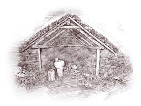
The raised roof in this construction allows for the heat to escape through a venting system in the roof.
